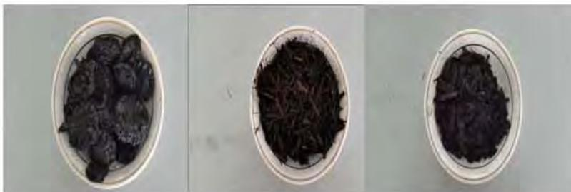
Figure 1. Processed activated carbons from: corn-cob, rice straw and sugarcane bagasse
